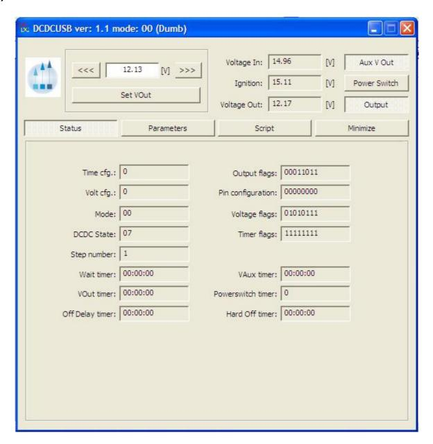
In this page you will find detailed description of several internal states and timers used in different modes: DUMB, AUTOMOTIVE, SCRIPT. Ex: this is useful when using the SCRIPT mode and testing the script programmed.
